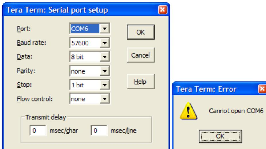
Note that the port number used to communicate with the SPB800E (COM6 in the figure above) might be different in some environments, so make sure to try another one if COM6 fails (see figure below)
