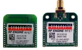
Each SNAP Engine combines a microcontroller, a radio, and an antenna. The antenna can either be an integral "F" antenna, or a mounting point for an external antenna. The SNAP Engines included in your EK2100 evaluation kit are RF100 SNAP Engines (also known as RF Engines), as pictured above at left. RF100 SNAP Engines communicate using 802.15.4 2.4 GHz radio signals.
