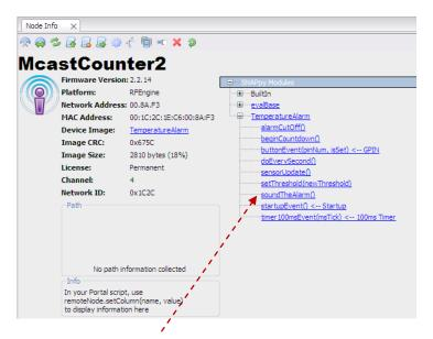
**Click** on the *soundAlarm()* function to test the buzzer. You should hear a long beep from the buzzer. (If you do not hear the beep, confirm that you have the buzzer's polarity correct in your installation.)
