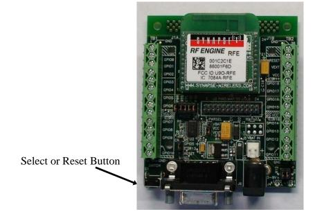
The Synapse SN171 Proto (prototyping) Board provides easy access to all 19 General Purpose Input/Output (GPIO) pins available on the RF100 SNAP Engine. Eight of these pins (GPIO 11-18) can also serve as analog inputs.
