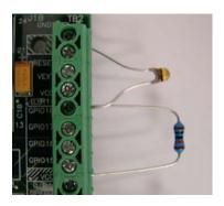
which pin. Again, a picture is worth a thousand words, so please refer to the figure for how the setup should look. Notice how you have to bend the legs of the thermistor to reach across several connector slots.
