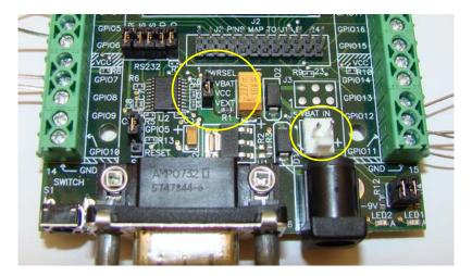
The jumper posts for this jumper are labeled "VBAT", "VCC", and "VEXT".
