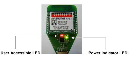
Power to this module is provided via a standard USB connection. This allows for the SNAPstick to be powered using a PC or other USB power source (such as an AC adaptor).
