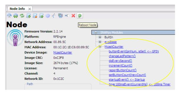
Here you can see the various functions defined in the "McastCounter.py" SNAPpy script. Like the built-in functions, these can also be directly invoked by clicking on them (and entering any needed parameters).
