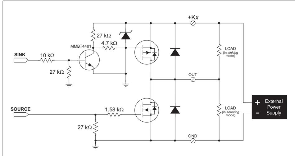
**Figure 10. BL4S200 High-Current Outputs**
