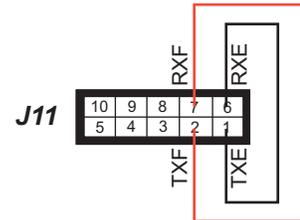
TxF and RxF become the flow control RTS and CTS. To test flow control, disconnect RTS from CTS while running this program. Characters should stop printing in the Dynamic C **STDIO** window and should resume when RTS and CTS are connected again
