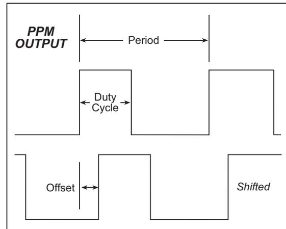
PWM and PPM outputs on the BL4S200 configurable I/O are configured using the `setPWM()` and `setPPM()` function calls. PWM and PPM outputs on the BL4S200 high-current outputs are configured using the `setPWM_H()` and `setPPM_H()` function calls.
