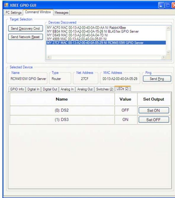
8. You are now ready to interface with the BL4S230 via the ZigBee protocol. Try pinging the selected device by clicking the “Send Ping” button.
