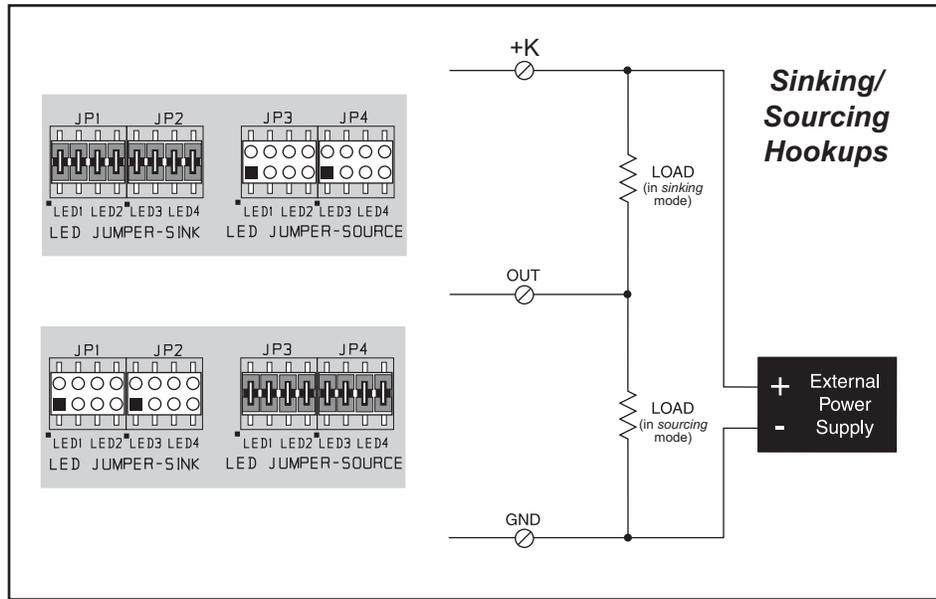
**Figure C-4. LED Output Indicators Sinking or Sourcing Configuration**
