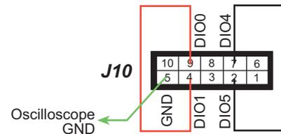
Once the connections have been made, compile and run this sample program. Change the offset and duty cycle for a given PPM channel via the Dynamic C **STDIO** window and watch the change to the begin and end counts measured on the input capture inputs. The PPM frequency can be changed in the `#define PPM_FREQ` line.
