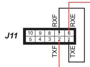
*BL4S210*—Connect TxB (pin 1 on connector J11) to RxB (pin 6 on connector J11) before compiling and running this sample program.
