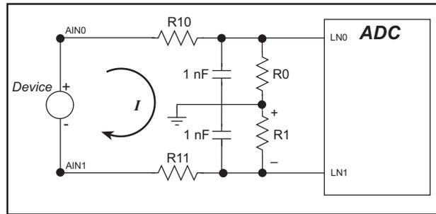
**Figure 9. Current Flow from Ungrounded or Floating Source**
