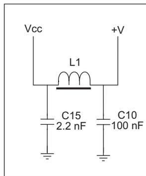
**Figure 11. Analog Supply Circuit**
