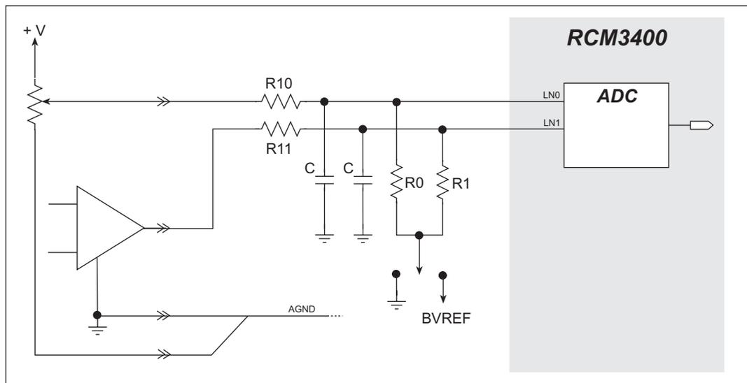
**Figure 8. Resistor Divider Network for Analog Inputs**
