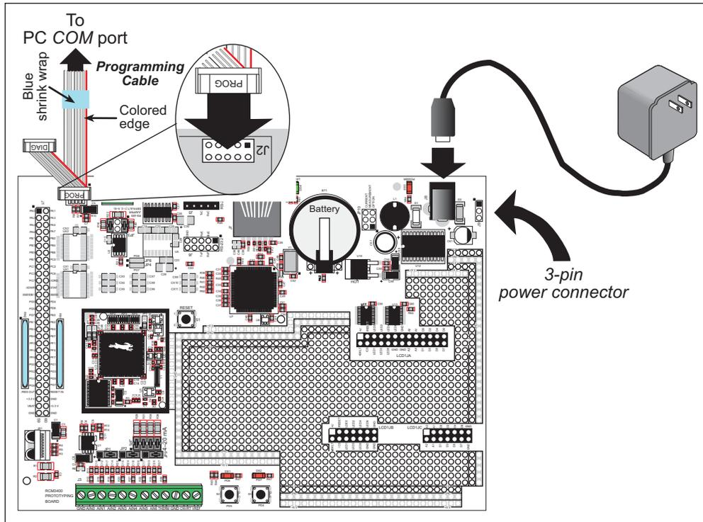
**Figure 3. Connect Programming Cable and Power Supply**
