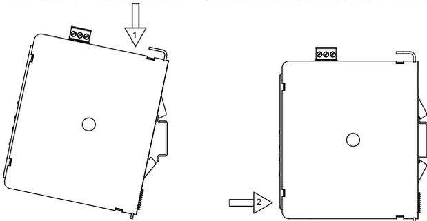
Figure 1 - Attach Data Station To DIN Rail
