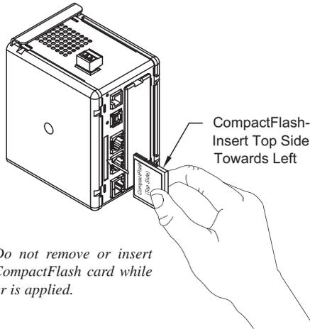
*Note: Do not remove or insert the CompactFlash card while power is applied.*
