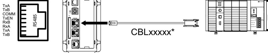
**WARNING:** Do **NOT** use a standard DH-485 cable to connect this port to Allen Bradley equipment.
