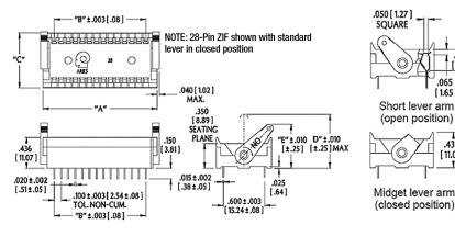
"A" = (NO. OF PINS PER ROW x 0.100 [2.54]) + 0.220 [5.588]"B" = (NO. OF PINS PER ROW -1) x 0.100 [2.54]
