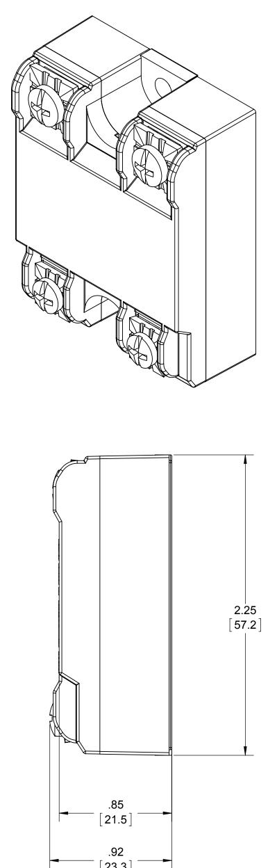
Tolerances: ± 0.02 in / 0.5 mm. All dimensions are in: inches [millimeters]
