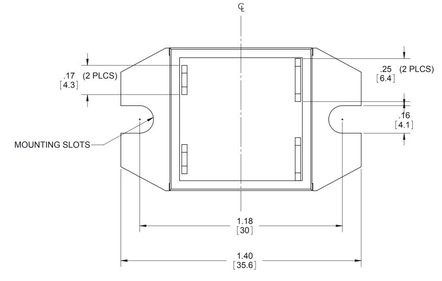
Tolerances: ± 0.02 in / 0.5 mm. All dimensions are in: inches [millimeters]
