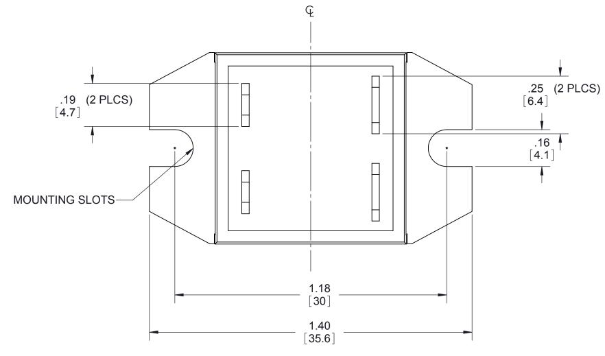
Tolerances: ± 0.02 in / 0.5 mm. All dimensions are in: inches [millimeters]
