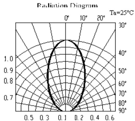
Typical Electro-Optical Characteristics Curves
