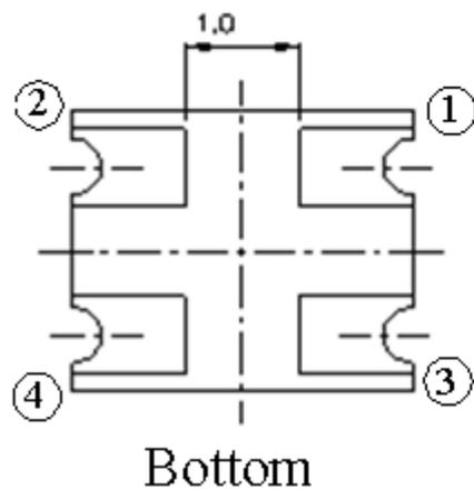
For reflow soldering (propose)
