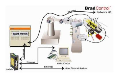
Contained in an IP67 rated housing, BradControl I/O modules can be machine mounted and are able to withstand areas where liquids, dust or vibration may be present. This makes them ideally suited for many applications including material handling equipment and automated assembly machinery.
