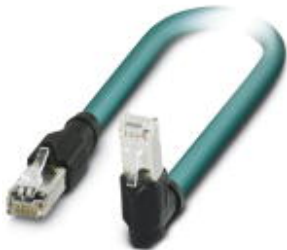
Patch cable, CAT5e, 4-pair, shielded, line, assembled at both ends with straight and angled RJ45/IP20 heads, length: 2 m
