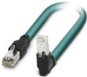
Patch cable, CAT5e, 4-pair, shielded, line, assembled at both ends with straight and angled RJ45/IP20 heads, length: 5 m
