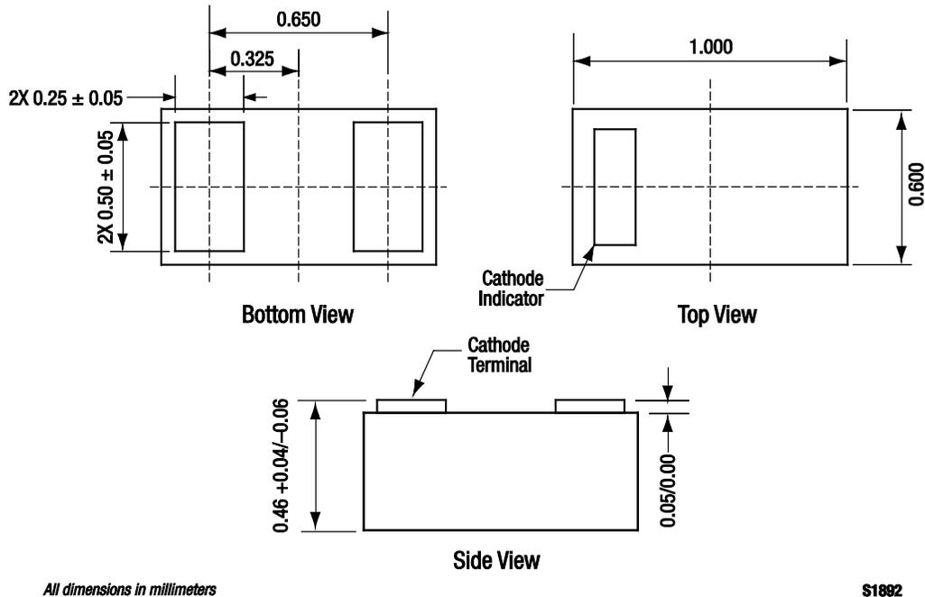
Figure 6. SOD-882 Package Dimensions
