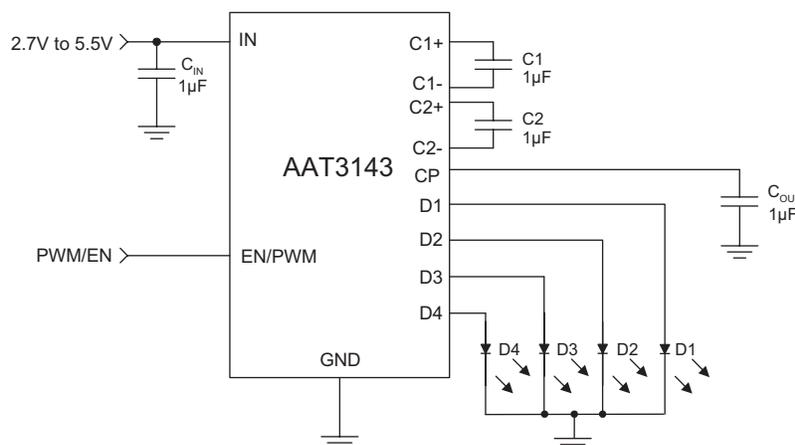
*High Efficiency 1X/1.5X/2X Charge Pump
