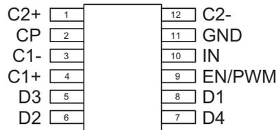
*High Efficiency 1X/1.5X/2X Charge Pump
