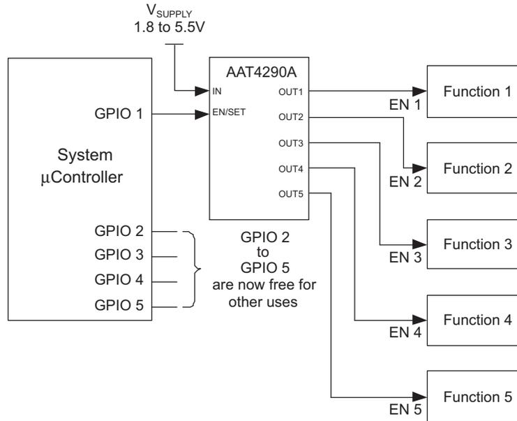
**Figure 1: GPIO I/O Expander**
