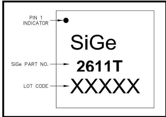
**Figure 4: SE2611T Branding and Pin 1 Location**
