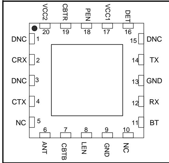
**Figure 2: SE2611T Pin out (Top View through Package)**
