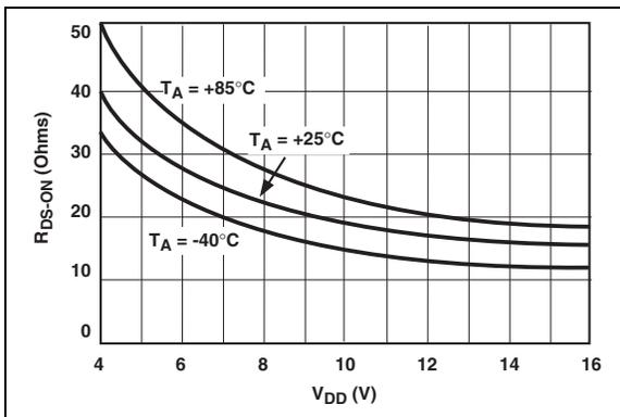
**FIGURE 2-3:** High-State Output Resistance vs. Supply Voltage.
