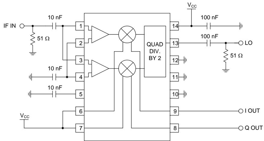
**Application Schematic - Modulator Configuration**
