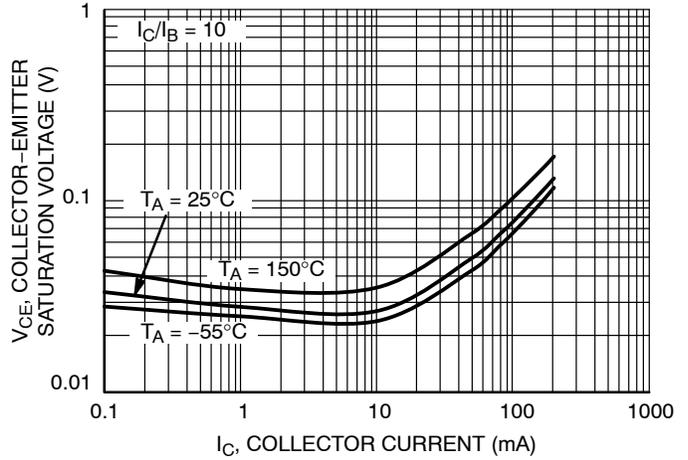
Figure 2. Collector Emitter Saturation Voltage vs. Collector Current
