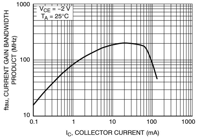
Figure 8. Current Gain Bandwidth Product vs. Collector Current
