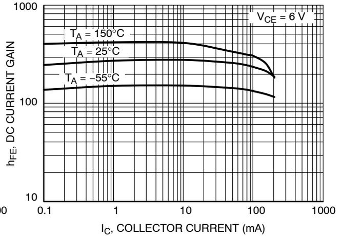
Figure 4. DC Current Gain vs. Collector Current
