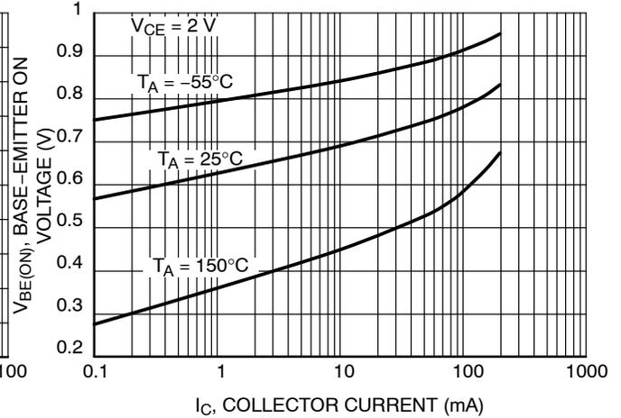
Figure 6. Base-Emitter Turn-ON Voltage vs. Collector Current
