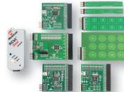
Provides a simple platform for developing a variety of capacitive touch sense applications using 16 and 32-bit PIC microcontrollers. The diagnostic tool
