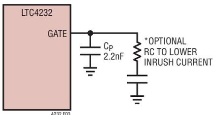
Figure 3. Compensation for Small C<sub>LOAD</sub>
