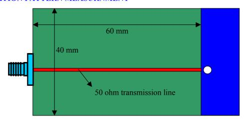
FR-4 PCB thickness = 0.8 mmThe length of transmission line = 1.35 mm ( depends on PCB thickness)
