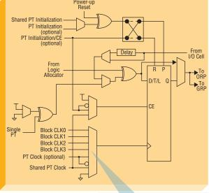
Flexible and efficient clock and control scheme ensures easy implementation with a variety of HDL coding styles.
