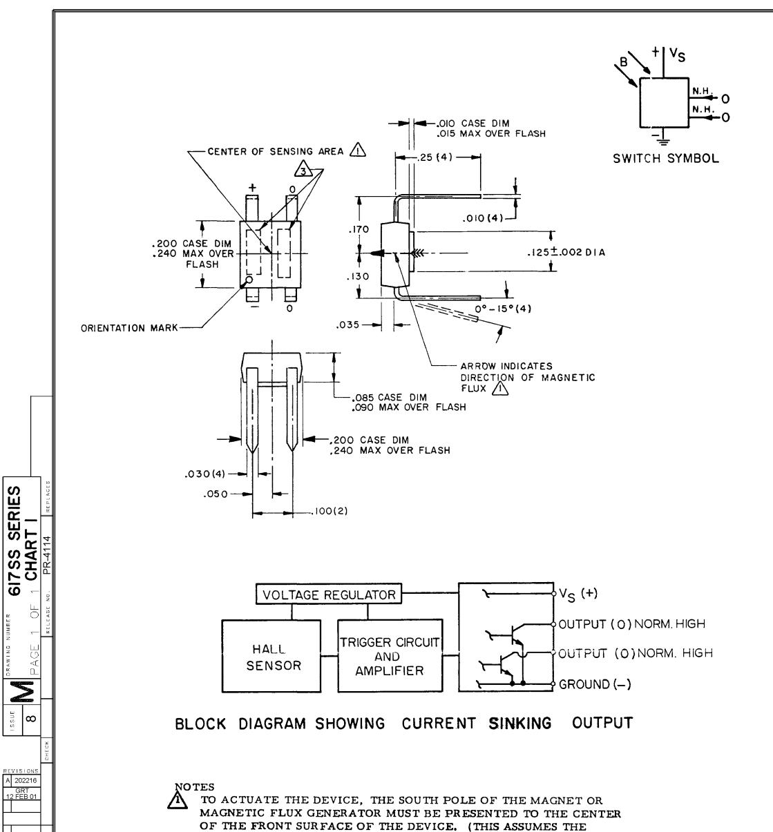
CONVENTION THAT THE DIRECTION OF THE EXTERNAL FLUX OF A MAGNET IS FROM THE NORTH TO THE SOUTH POLE OF THE MAGNET.)
