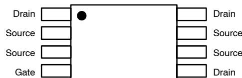
Figure 2. Pinouts for Single Die TSSOP
