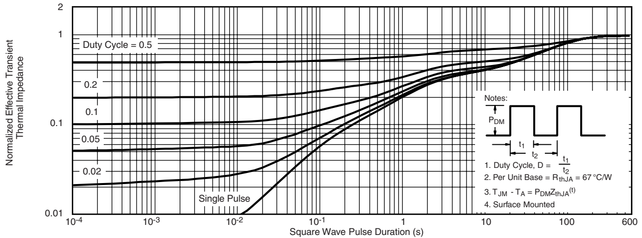
Normalized Thermal Transient Impedance, Junction-to-Ambient
