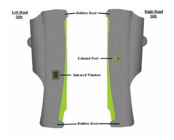
Exhaust Port Port for connection of Exhaust Adaptor
