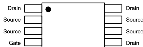
Figure 2. Pinouts for Single Die TSSOP
