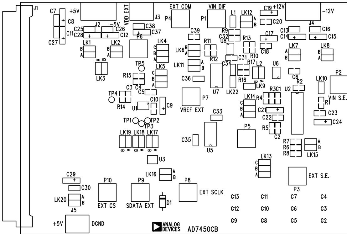
Figure 8. AD7450 Evaluation Board Component Placement Drawing.
