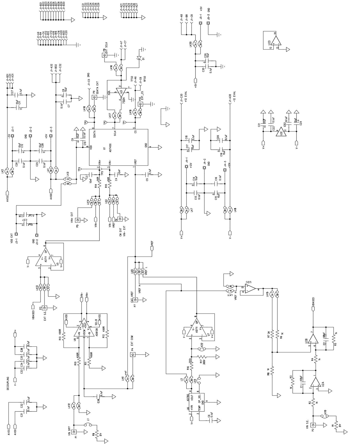
Figure 5. AD7450 Evaluation Board Circuit Diagram
