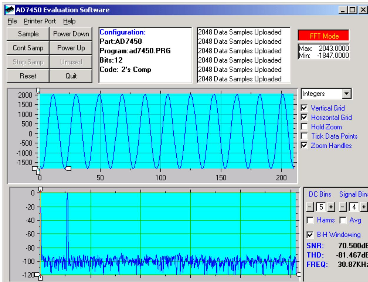
Figure 2. AD7450 Main Screen - FFT Mode
