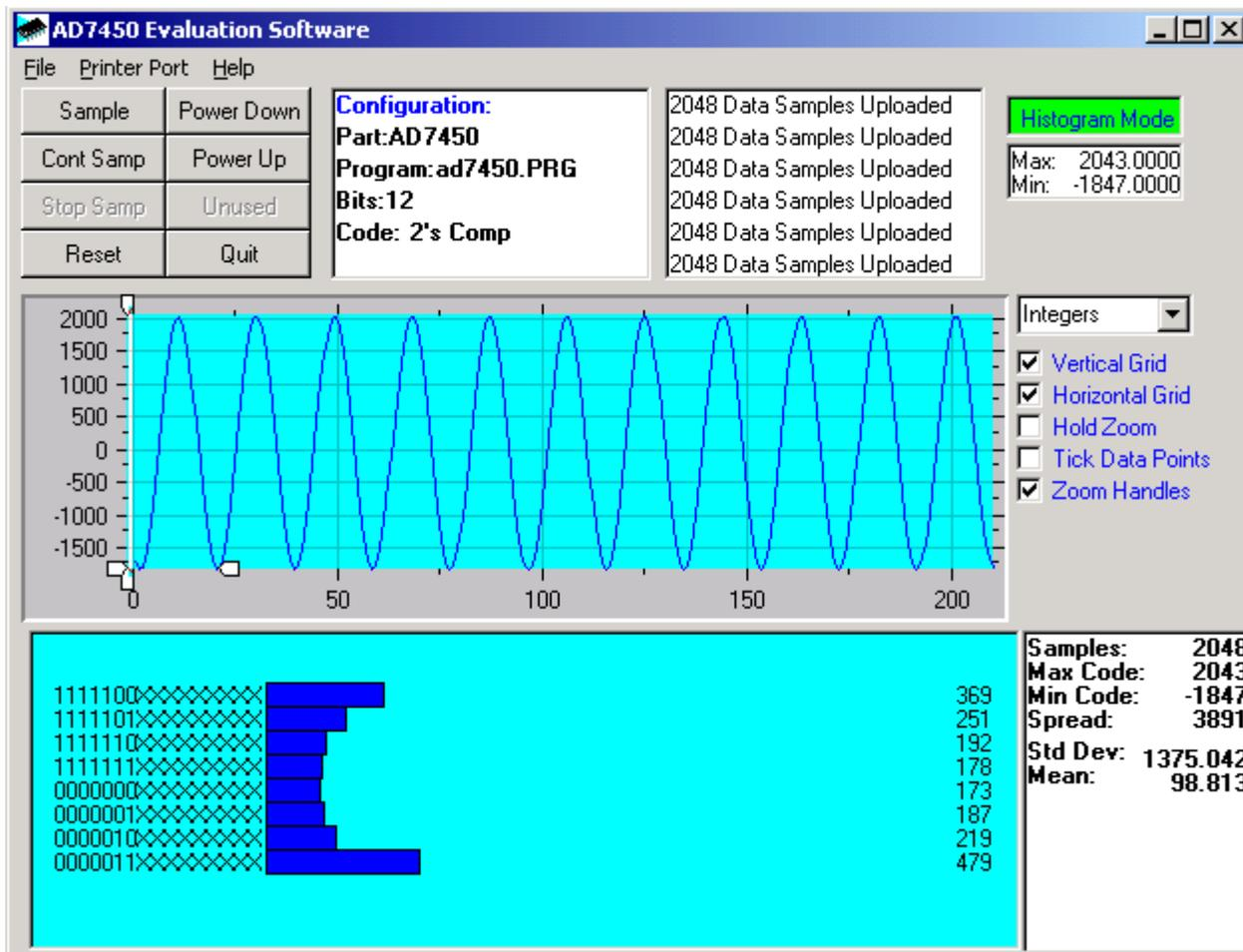
Figure 3. AD7450 Main Screen - Histogram Mode
