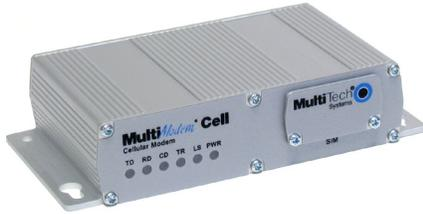
The MultiModem® Cell GPRS cellular modem offers standards-based quad-band GPRS performance. This ready-to-deploy, standalone modem provides wireless data communication and integrates seamlessly with virtually any application. It is available with a broad range of interface options including RS-232/RS-422 and USB to cover all of your application needs. The MultiModem Cell cellular modem is based on industry-standard open interfaces and can be desktop or panel mounted.
