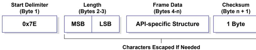
MSB = Most Significant Byte, LSB = Least Significant Byte
