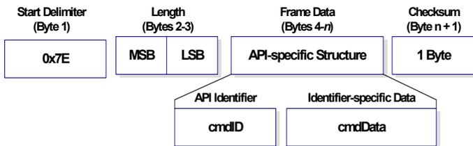
The cmdID frame (API-identifier) indicates which API messages will be contained in the cmdData frame (Identifier-specific data). Note that multi-byte values are sent big endian. The XBee modules support the following API frames:
