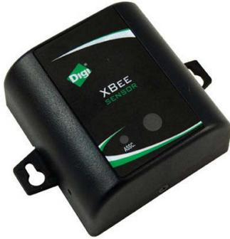
The XBee Sensor family is a group of XBee-enabled, battery-powered sensors incorporating an RF module. As a part of Digi's Drop-in Networking solutions, XBee-enabled sensors read real-time data from sensors such as temperature, humidity, and light.
