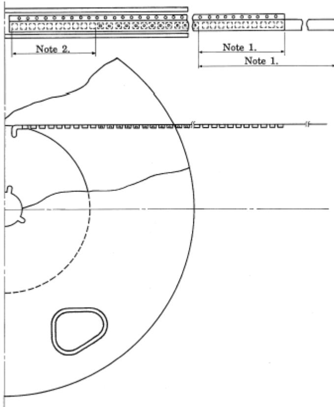
Note 1 : The leader portion shall consist of cover tape minimum length of 300 mm and a piece of carrier tape with empty portion of 100 mm minimum.
