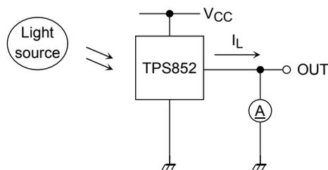
Note 5: Switching time measurement method
