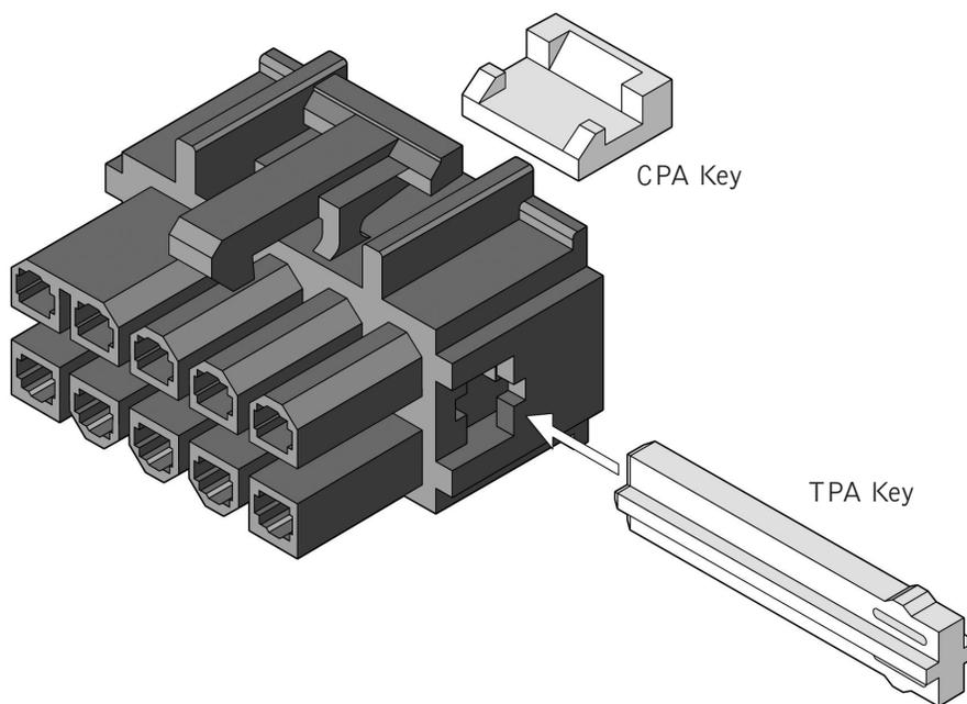
\*Current - 13.0A max. per circuit when header is mated to a receptacle loaded with 45750 series terminals crimped to 16 AWG wire. See Molex product specification PS-45750-001 for additional current derating information
