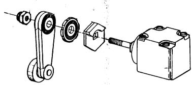
ADJUSTABLE TO OPERATE CLOCKWISE, COUNTER-CLOCKWISE, OR IN BOTH DIRECTIONS.
