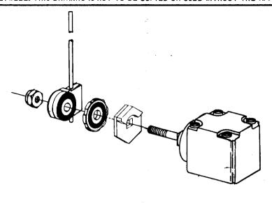
ADJUSTABLE TO OPERATE CLOCKWISE, COUNTER-CLOCKWISE, OR IN BOTH DIRECTIONS.
