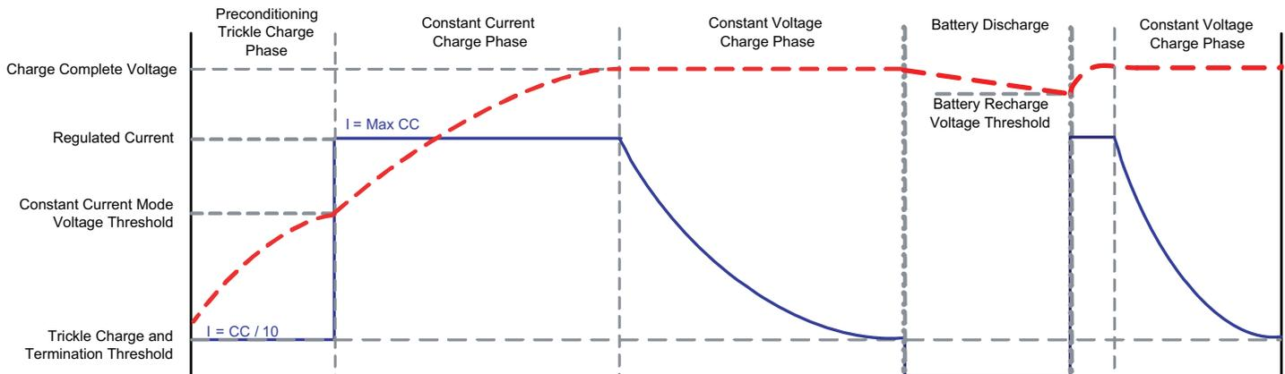
**Figure 1: Current vs. Voltage Profile During Charging Phases.**
