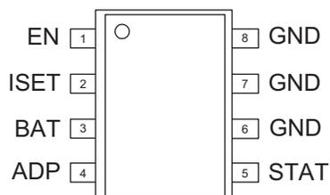
*USB Port or AC Adapter Li-Ion/Polymer Battery Charger*
