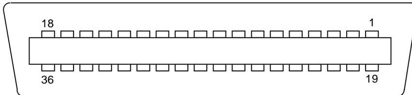
Fig. 3: 36-way Centronics (P2) Pin Configuration
