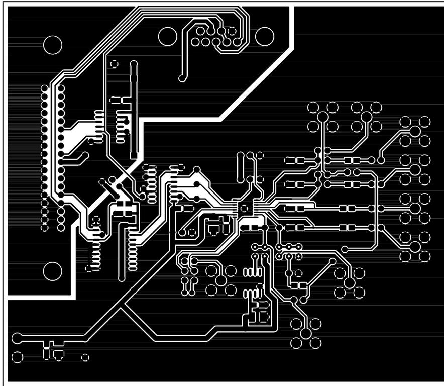
Fig. 23. The Evaluation Board Component Side Artwork
