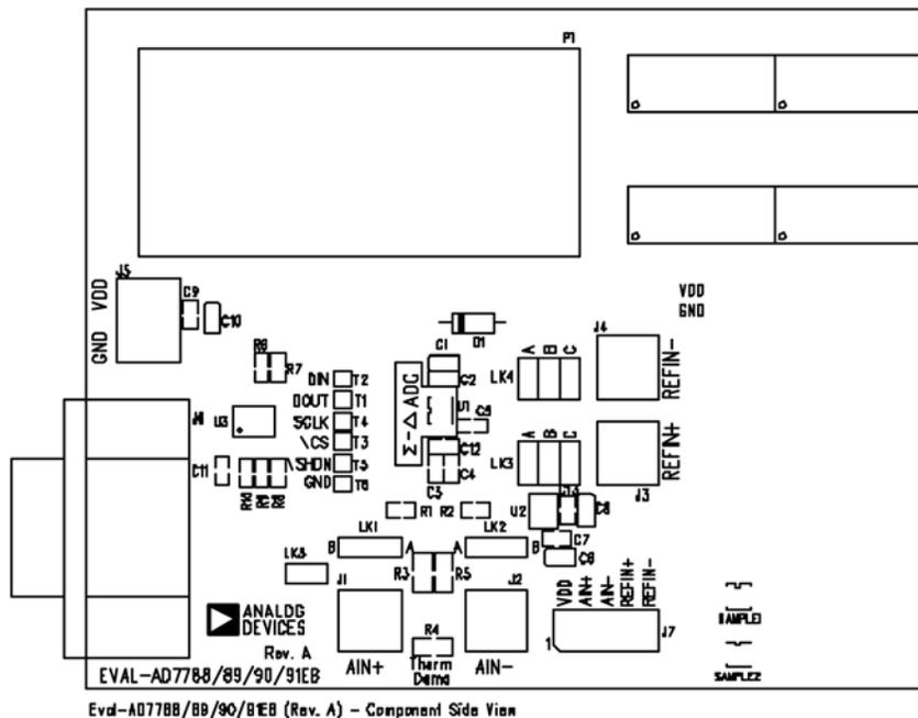
Figure 13. Evaluation Board Component Layout Diagram
