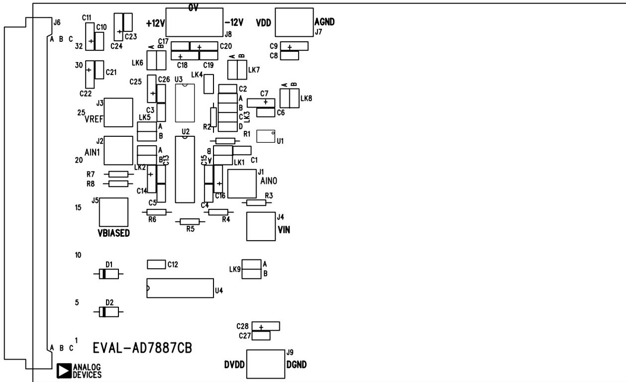
Figure 8. AD7887 Evaluation Board Component Placement Drawing.
