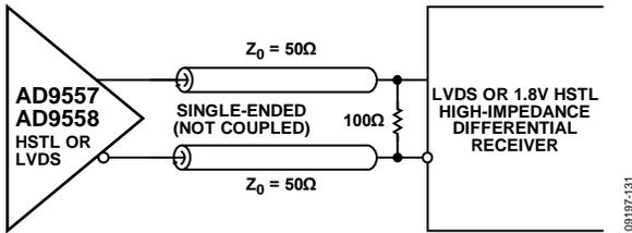
Figure 31. DC-Coupled LVDS or HSTL Output Driver
