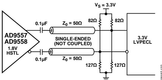
Figure 32. Interfacing the HSTL Driver to a 3.3 V LVPECL Input
