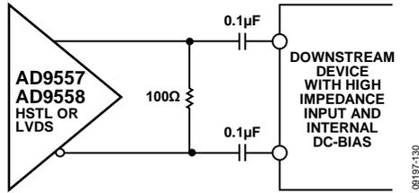
Figure 30. AC-Coupled LVDS or HSTL Output Driver
