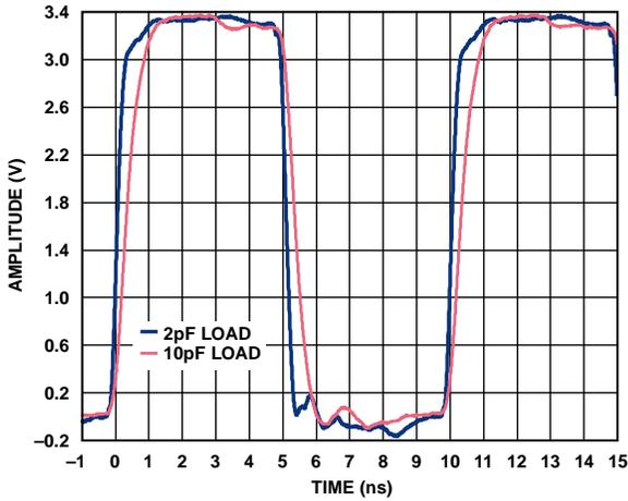
Figure 25. Output Waveform, 3.3 V CMOS (100 MHz, Strong Mode)
