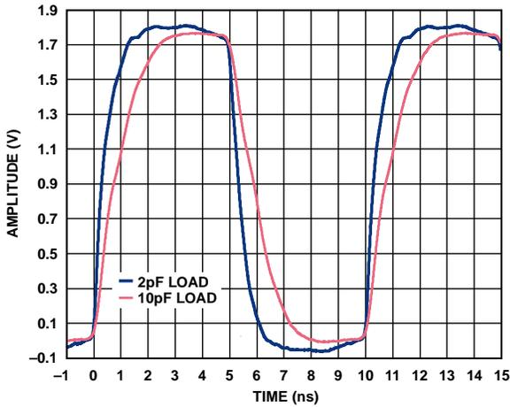
Figure 26. Output Waveform, 1.8 V CMOS (100 MHz)
