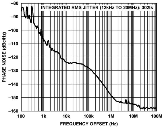
Figure 7. Absolute Phase Noise (Output Driver = 3.3.V CMOS),
