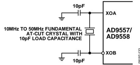
Figure 33. System Clock Input (XOA, XOB) in Crystal Mode
