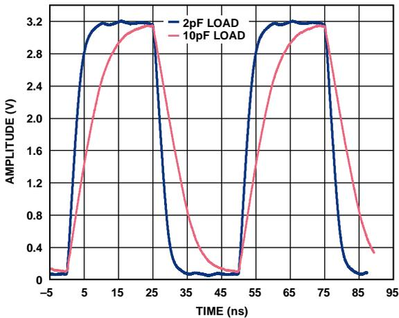
Figure 27. Output Waveform, 3.3 V CMOS (20 MHz, Weak Mode)
