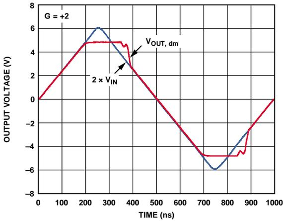
Figure 43. Output Overdrive Recovery,  $G = 2$
