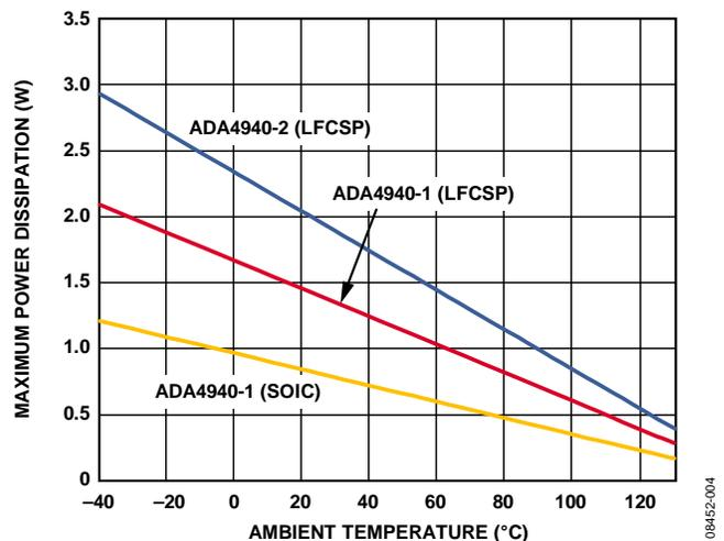
Figure 3. Maximum Safe Power Dissipation vs. Ambient Temperature
