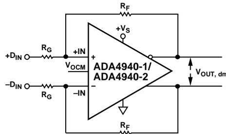
Figure 64. ADA4940-1/ADA4940-2 Configured for Balanced (Differential) Inputs
