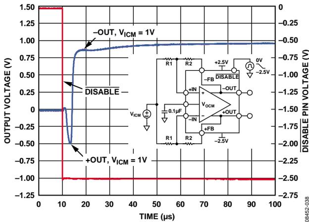
Figure 45.  $\overline{\text{DISABLE}}$  Pin Turn-Off Time
