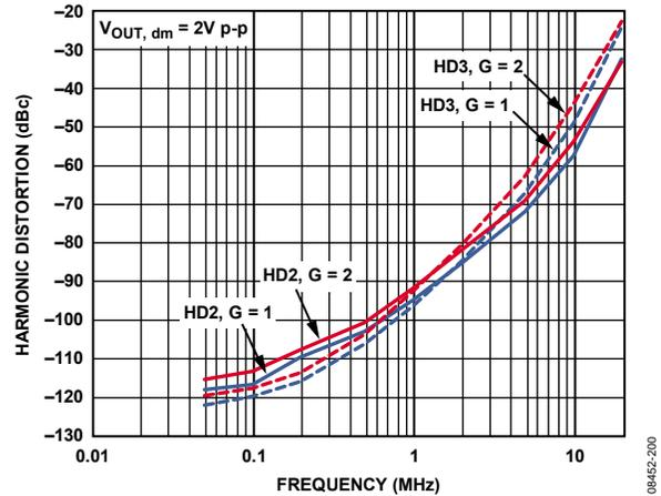
Figure 28. Harmonic Distortion vs. Frequency vs. Gain (SOIC)
