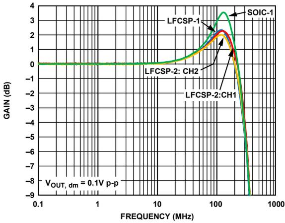
Figure 13. Small Signal Frequency Response for Various Packages
