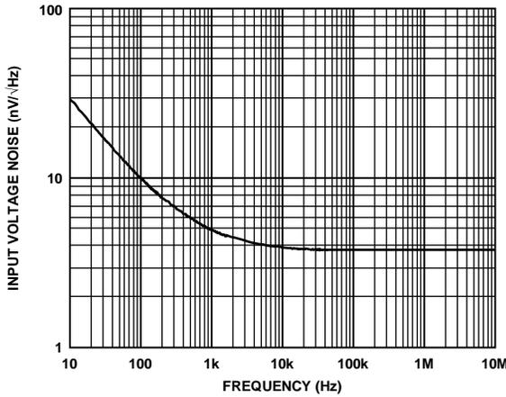
Figure 44. Voltage Noise Spectral Density, Referred to Input
