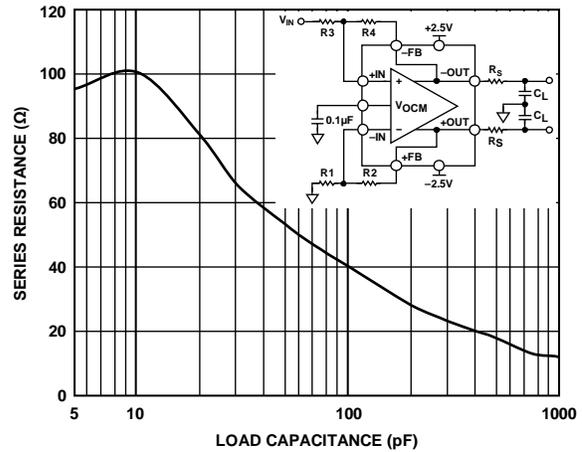
Figure 71. Capacitive Load vs. Series Resistance (LFSCP)
