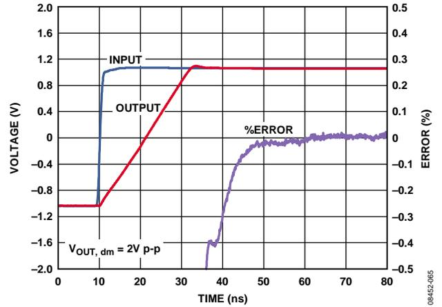
Figure 46. 0.1% Settling Time
