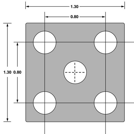
Figure 75. Recommended PCB Thermal Attach Pad Dimensions (mm)
