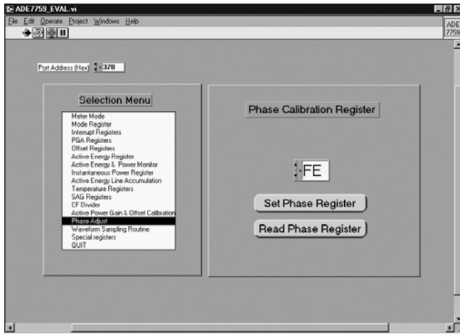
Figure 14. Writing to the PHCAL Register to Correct Phase Error
