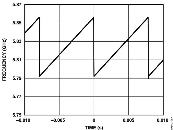
Figure 8. Sawtooth Waveform, PFD = 32 MHz, INT = 181, FRAC = 0, DEV Offset = 4, DEV Word = 20972, Step Word = 200, CLK<sub>2</sub> Divider = 10, CLK<sub>1</sub> Divider = 125
