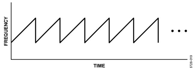
Figure 33. Sawtooth Ramp
