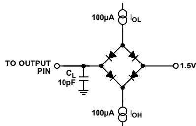
Figure 4. Load Circuit for MUXOUT Timing, C = 10 pF
