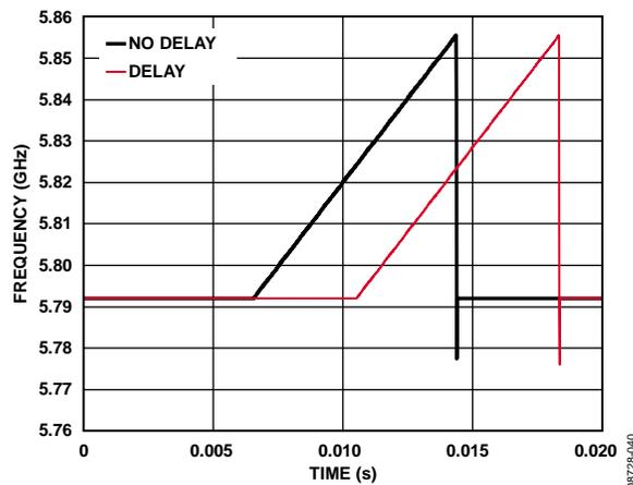
Figure 10. Delayed Start of Triangular Burst, PFD = 32 MHz, INT = 181, FRAC = 0, DEV Offset = 4, DEV Word = 20972, Step Word = 200, CLK<sub>2</sub> Divider = 10, CLK<sub>1</sub> Divider = 125, DEL Start Word = 1000
