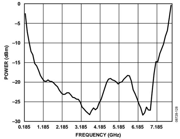
Figure 14. RF IN Sensitivity-Average Over Temperature and V<sub>DD</sub>
