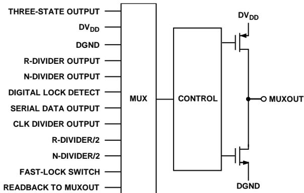
Figure 20. MUXOUT Schematic
