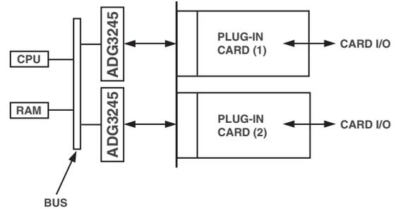
Figure 12. ADG3245 in a Hot Plug Application
