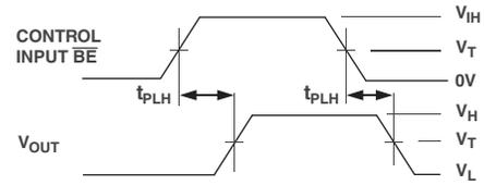
Figure 2. Propagation Delay
