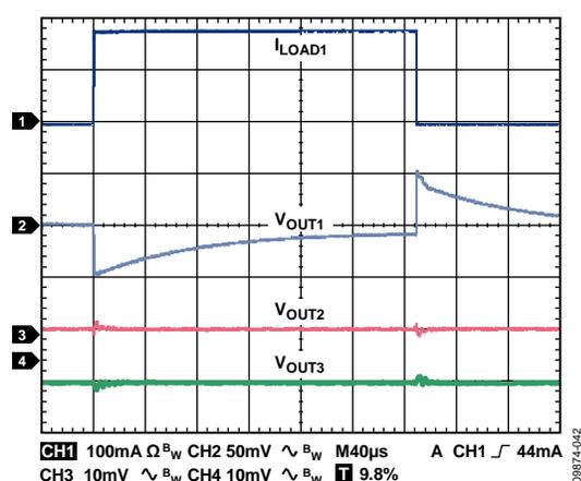
Figure 42. Output Transient Response,
