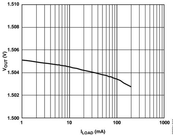
Figure 10. Output Voltage vs. Load Current
