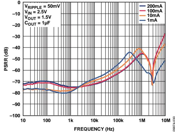
Figure 30. Power Supply Rejection Ratio vs. Frequency, 1.5 V
