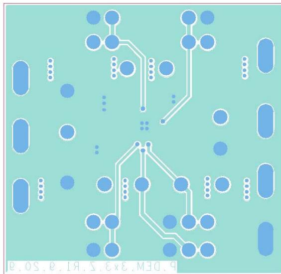
Figure 52. Example of PCB Layout, Bottom Side
