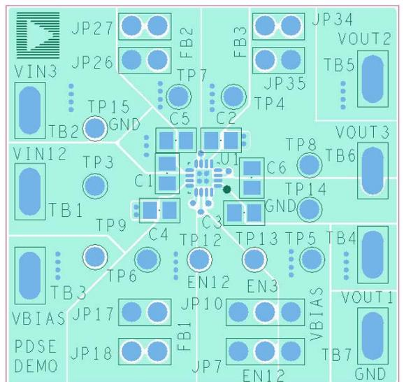
Figure 51. Example of PCB Layout, Top Side
