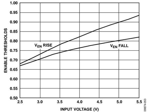
Figure 45. Typical  $EN_x$  Pins Thresholds vs. Input Voltage
