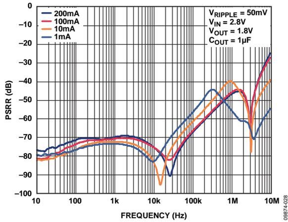
Figure 28. Power Supply Rejection Ratio vs. Frequency, 1.8 V
