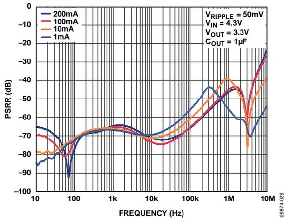
Figure 29. Power Supply Rejection Ratio vs. Frequency, 3.3 V
