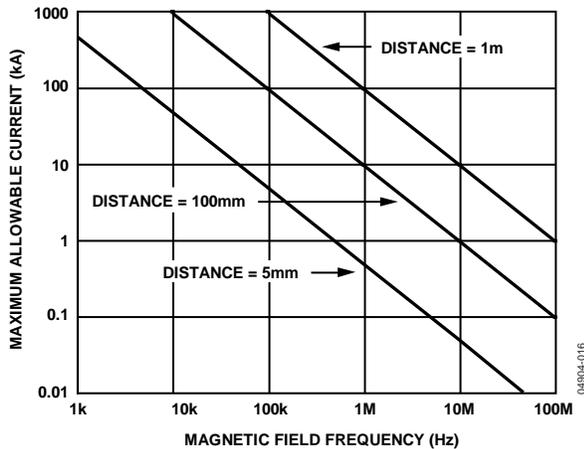
Figure 16. Maximum Allowable Current for Various Current-to-ADuM131x Spacings
