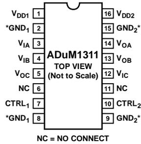
\*PIN 2 AND PIN 8 ARE INTERNALLY CONNECTED. CONNECTING BOTH TO GND<sub>1</sub> IS RECOMMENDED. PIN 9 AND PIN 15 ARE INTERNALLY CONNECTED. CONNECTING BOTH TO GND<sub>2</sub> IS RECOMMENDED.
