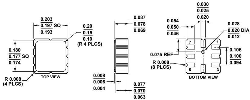
Figure 18. 8-Terminal Ceramic Leadless Chip Carrier [LCC]
