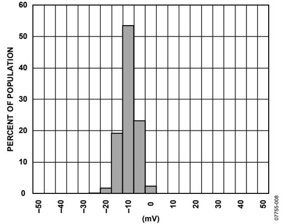
Figure 9. Y-Axis Zero g Bias Deviation from Ideal at 25°C
