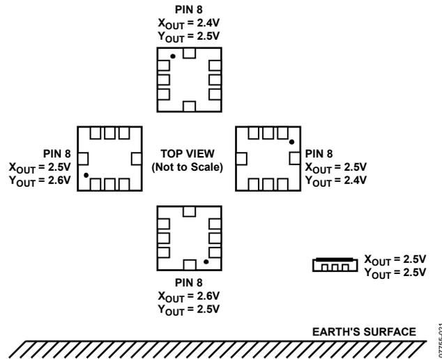
Figure 17. Output Response vs. Orientation
