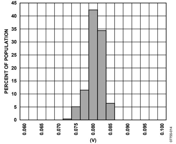
Figure 15. Y-Axis Self-Test Response at 25°C
