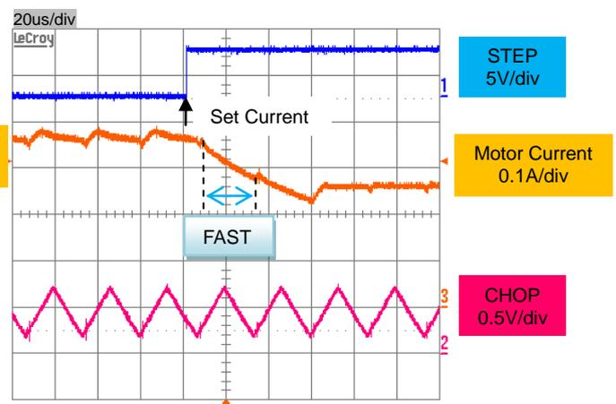
Figure 37. Constant current control waveform (Decreasing direction)
