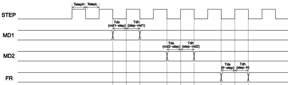
TstepH/TstepL: Clock H/L pulse width (min 500ns)
