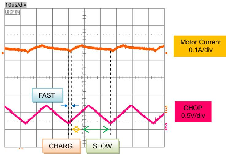
Figure 35. Constant current control waveform (Stationary state)
