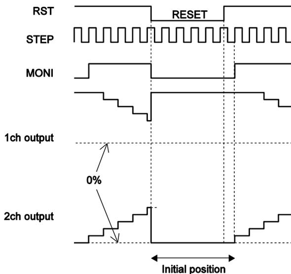
Figure 21. Reset function timing chart
