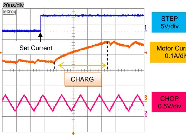
Figure 36. Constant current control waveform (Increasing direction)
