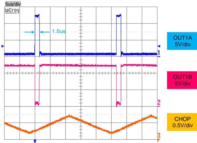
From the above Fig. , the blanking time appears to be  $1.5 \mu s$ . However, since the mode shifts from charge (blanking time), OFF, to DECAY, the actual blanking time is obtained as follows:
